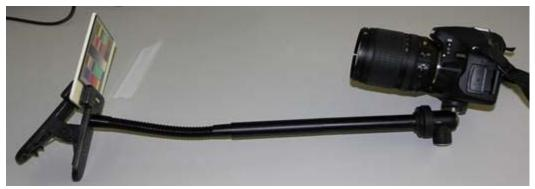
Figure B.1: Example fixture used for the side-by-side image capture method.
