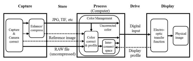
Figure 1: Functional flow diagram of a generic digital color image process, from image capture to its display. The concept of the reference image is used for workflows were color correction are applied.
