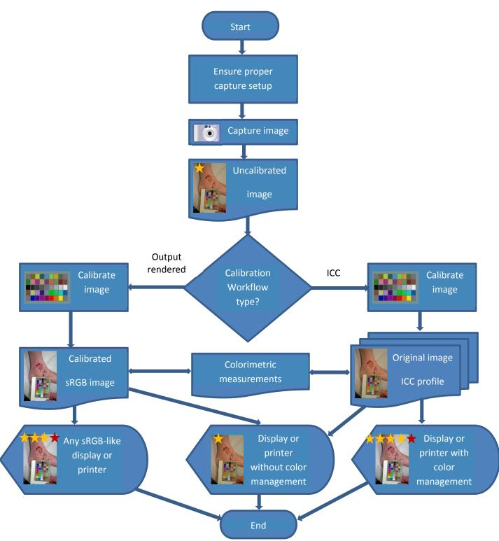
Figure 7: Functional flow diagram of the color correction process, with either direct outputreferred rendering or the use of ICC profiles.
